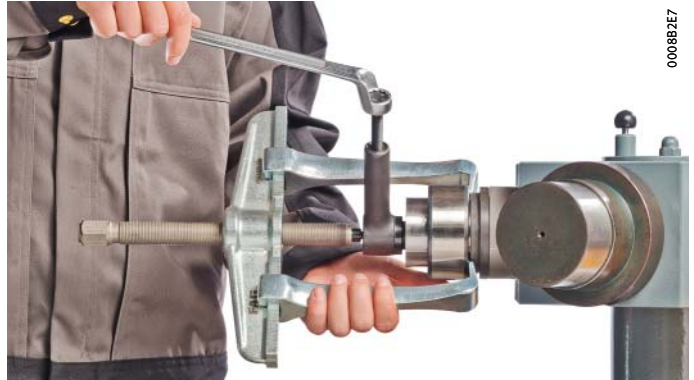
Figure 3 Use of the hydraulic pressure tool PULLER-SUPPORT
