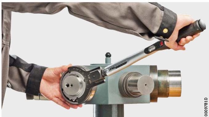
Figure 3 Use of the double hook wrench LOCKNUT-DOUBLEHOOK
