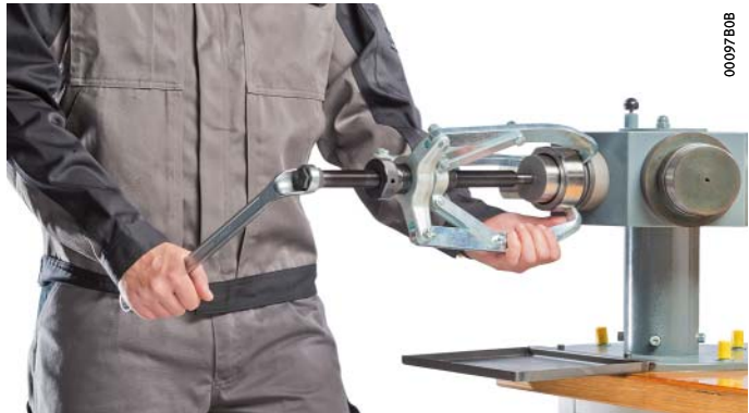
Figure 2 Use of the three-arm extractor PULLER-3ARM
