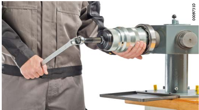
Figure 4 PULLER-SPECIAL: extraction of the bearing
