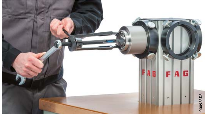
Figure 1 Use of the internal extractor PULLER-INTERNAL
