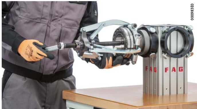
Figure 2 Use of the three-section extraction plate PULLER-TRISECTION
