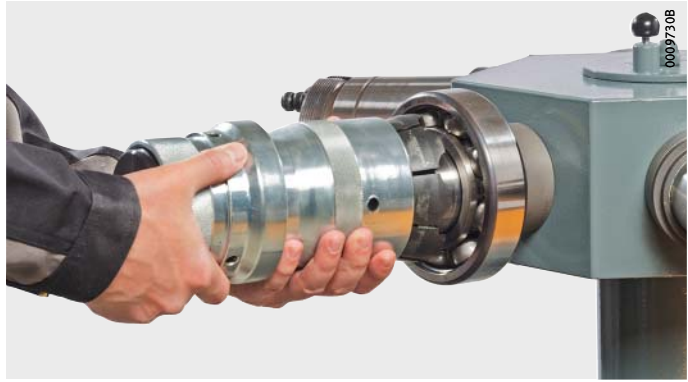
Figure 2 PULLER-SPECIAL: positioning on the bearing
