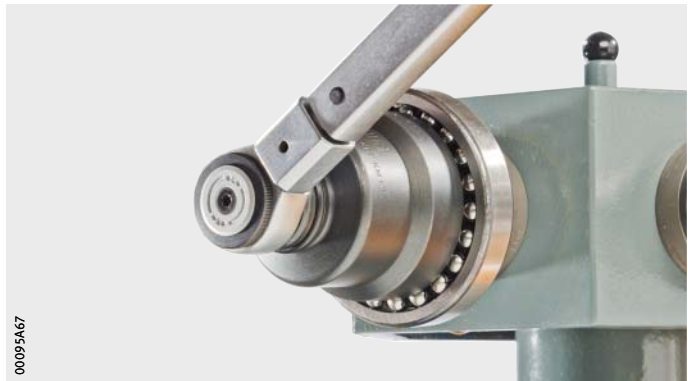
Figure 2 Use of the socket LOCKNUT-SOCKET
